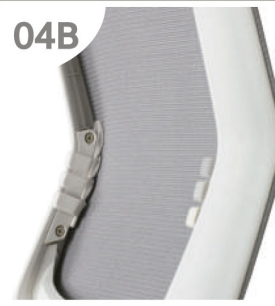
Lumbar support (Lever type) The pair of lever in the backrest are simultaneously adjusted by user. It is possible to adjust to the optimum state according to the body type of user.
